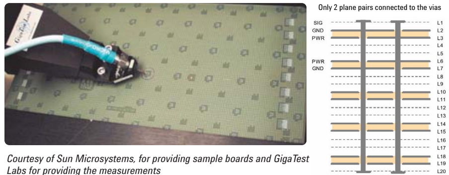
Figure 38. Probing the the PCB structure and layer layout
